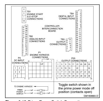
Figure 6-13 Prime Power Switch Connections
